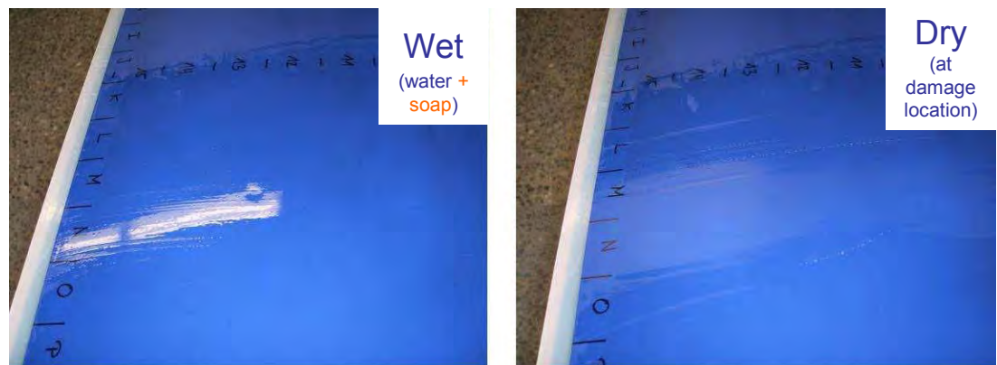
Figure 60: Surface wetting, to improve detectability of dents on matt surface.
